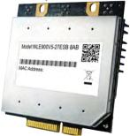
With 700Mhz high performance CPU, WPJ558 provide sufficient processing power to attain 802.11ac speeds up to 1300Mbps at 5Ghz paired with 3x3 MIMO WLE900V5-27 leveraging Nextgen high bandwidth 802.11ac transfers
